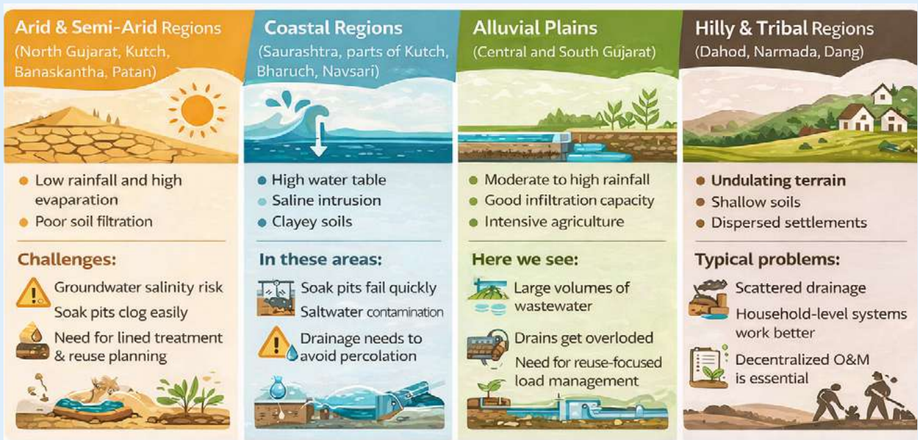
Figure 16: An example of Gujarat to show how Greywater planning can be done based on hydrogeological parameters of the state – A guide to say ‘why one size solution does not fit for all’.
